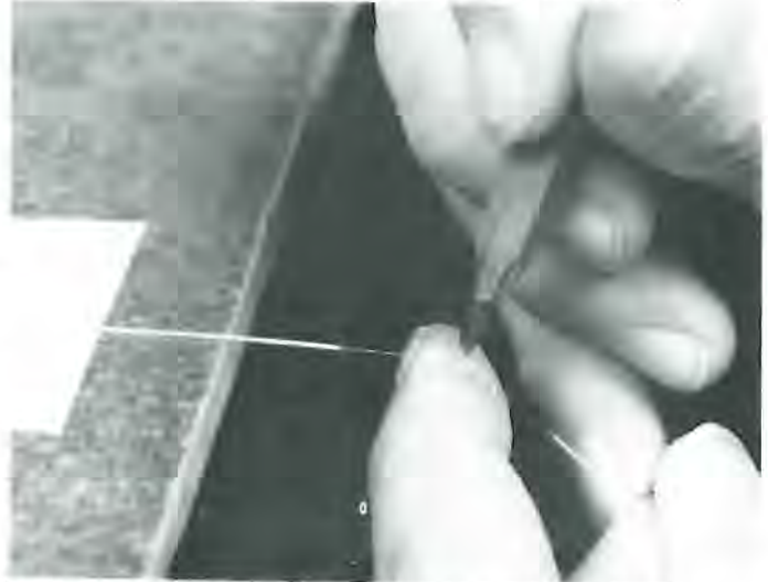
Fig 3 —To avoid scoring the glass when removing the tough jacket material from an ITT cable, keep the blade angle low.
