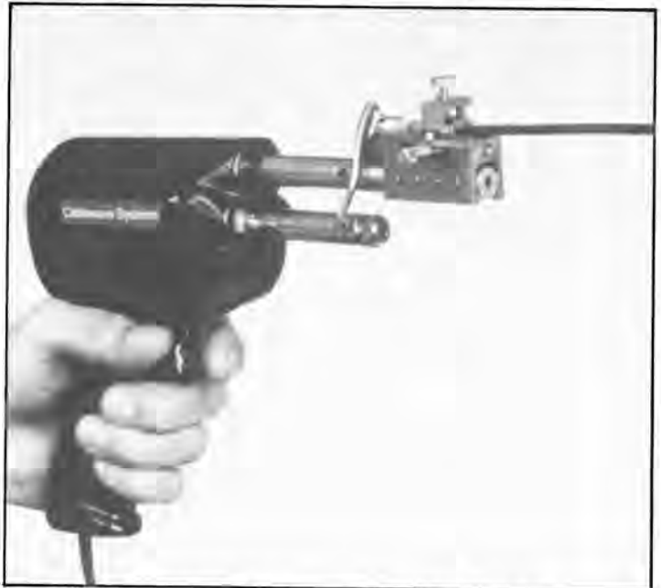
By melting the fiber into the connector nosepiece with this semi-automatic tool, you can install Cablewave Systems' connectors without ever handling the delicate cable fiber. Fiber alignment is also independent of core concentricity.
